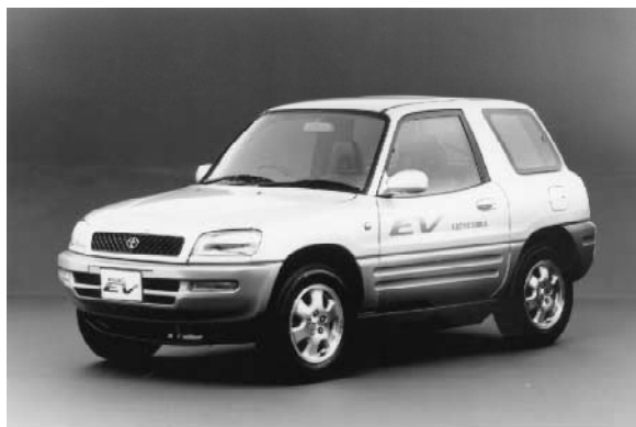
Fig. 3. The electric vehicle (TOYOTA RAV4L) powered by a Ni–MH battery, which is scheduled for commercialization in the autumn of 1996 [22]. Curb weight: 1410 kg, Maximum speed: 125 km h -1 , running distance per charge: 215 km (10–15 mode).
